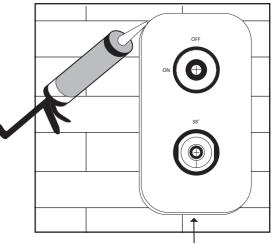
Leak detection channel
