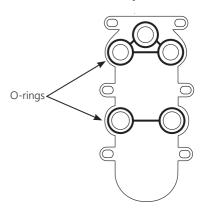
7. Place the valve body into the ARMERA dock and use the locating lugs to set the body in the correct position. Secure the valve body in position using the fixing screws. Ensure that screws are tightened sufficiently for the valve body to create a water tight seal with the ARMERA dock.
