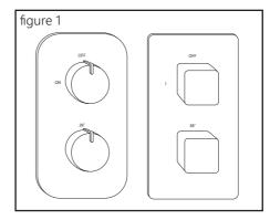
Use a thermometer to test the water temperature from one of the outlets. Adjust the temperature by turning the temperature control handle clockwise or anti-clockwise until 38°C is achieved. Remove the handle and re-attach it so it is aligned as shown in figure 1.
