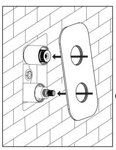
11. Seal the plate to the tiles using silicone sealant. Ensure to leave the channel at the bottom of the plate free of silicone. If a leak ever occurs in the valve, this channel will allow water to escape alerting you of a problem.
