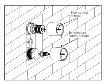
10. Push the backplate onto the flow control and temperature control shrouds.
