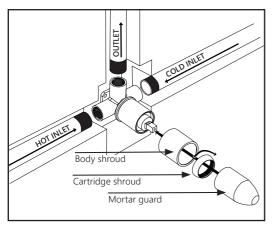
5. Offer the valve body up to the wall onto which it will be fixed and ensure it is level. Mark the fixing points and then fix the valve body securely to the wall.
