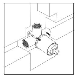
7. Fix the finished wall in place then remove the mortar guard and slide the cover plate onto the body shroud.
