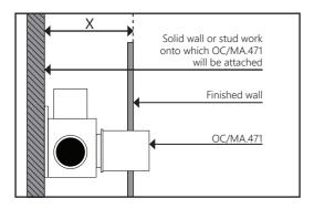
6. Connect all inlets and outlets. Turn on the water supply to test all pipework for leaks. Next, slide on the body shroud and secure it in place by screwing on the cartridge shroud. Turn the water supply off and fit the mortar guard to protect the valve during the next stages of insulation.
