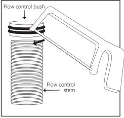
Ensure to only cut the end of the stem onto which the flow control bush is fitted. Do not cut the end that screws onto the valve body!
