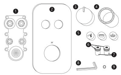
\* 2 outlet valve (IN.332.60) is shown for illustrative purposes only. For 1 outlet valve (IN.331.60) only 1 flow control bush and 1 flow control stem will be present.
