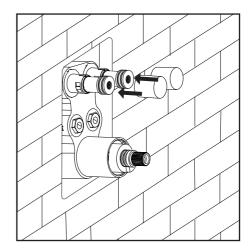
11. Push the backplate onto the flow control buttons and temperature control shroud.
