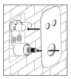
12. If the flow control buttons protrude too far out of the plate, remove the flow control buttons and the backplate. Unscrew the flow control bush from the flow control stem and cut down the flow control stem to the desired length. Reassemble back into valve body and replace the back plate and flow control buttons.
