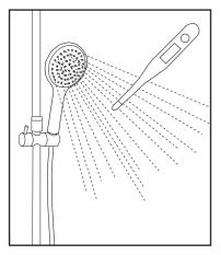
The valve has been calibrated so that 38°C is achieved with the thermostatic control handle positioned as in below diagram. If water temperature is higher or lower than 38°C, please follow the instructions for recalibrating the thermostat.
