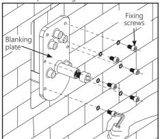
6. Check to ensure that the o-rings are firmly secured in the back of the valve body. If the o-rings are damaged or not seated correctly, the valve body will not seal with the ARMERA dock and leaks may occur.
