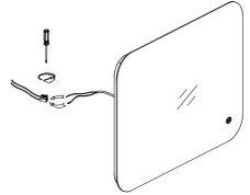
This product is manufactured to class 2 category and should be connected to the mains as shown here:
