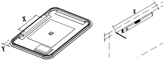
2. Use a suitable drill bit to drill holes then insert rawl plugs. The bracket can then be fixed to the wall with the screws. If mounting the product to plasterboard walls, appropriate fixings should be used.
