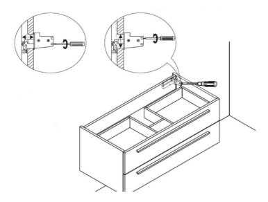
7. After any adjustment of the unit has been made, the basin can be fitted to the unit by applying a bead of silicone between the unit and the basin to provide a seal. A bead of silicone should also be applied to the top back edge of the basin where it meets the wall.
