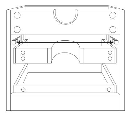
2. Decide the desired height of the basin unit and mark a horizontal line on the wall. Use the measurement made in step 1 to mark the position of the fixing brackets on the wall ensuring that when the unit is attached to the brackets, the whole bracket fits inside the unit.
