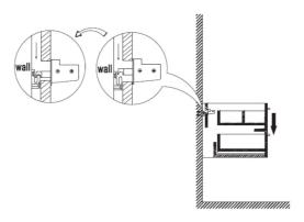
6. If any adjustment forward, backward, up, or down is required this is possible via the fitted adjusters on the inside of the unit.
