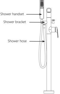
13. Turn on the water supply and check for leaks with the mixer in the on and off positions and water diverted to the spout and handset.
