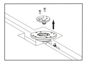
9. Push the inlet pipes that protrude from the base of the body into the hot and cold outlets on the fixing seat. Take care not to damage the rubber O-rings on the inlet pipes.
