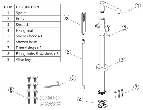
Before installation, please ensure that the plumbing system has been fully flushed to remove dirt and debris.
