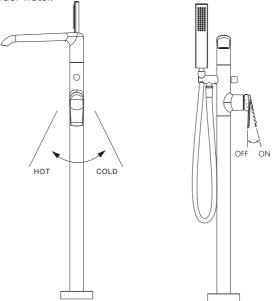
15. To operate the shower handset, turn on the water flow and pull the diverter knob away from the body. The diverter knob can be locked in position by rotating it clockwise by 90 degrees.
