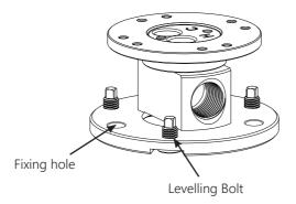
7. Connect the hot and cold water supplies to the fixing seat. Hot is marked with an "H" and cold with a "C".
