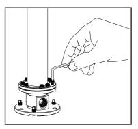
11. Taking care not to damage the rubber O-rings, push the spout into the body and secure in position by tightening the grub screw
