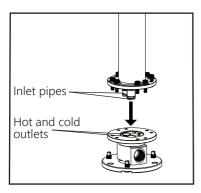
10. Rotate the body so that the spout will be facing the correct direction when it is attached, then secure the body to the fixing seat using the fixing bolts and washers. 8 bolts and washers are provided. For a firm fixing please use a minimum of 6 bolts.
