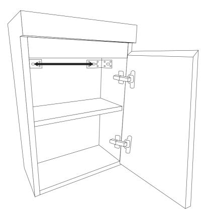
2. Decide the desired height of the basin unit and mark a horizontal line on the wall (recommended height is shown below). Use the measurement made in step 1 to mark the position of the fixing holes on the wall.
