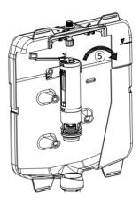
6. The volume of full flush can be adjusted by moving the flush adjustment slider up to decrease volume or down to increase volume. The volume of half flush can be adjusted by twisting the blue flush adjuster and sliding it up to decrease the volume and down to increase it. Once desired volume is achieved, the blue flush adjuster should then be twisted back into the locked position.
