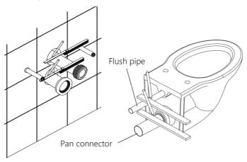
3. Cut the flush pipe and pan connector to the correct length.
