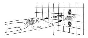
9. Insert the allen key (A) into the seat cover hole in the toilet pan. Use it to tighten the grub screws (E), securing the toilet pan in position.
