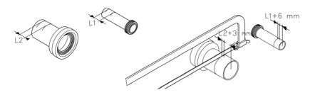
4. Make a chamfer on the outer face of the flush pipe and pan connector and apply silicon grease to the inner face of the pipes in the wall.
