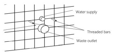
2. Mark the correct lengths for the flush pipe and pan connector (supplied with the concealed cistern).
