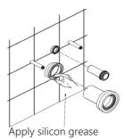
5. Cut the threaded bars on the wall to a length of 38mm then screw part B onto the threaded bars ensuring the machined groove faces upwards.
