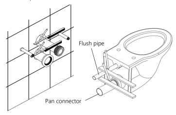
3. Cut the flush pipe and pan connector to the correct length.
