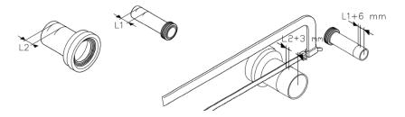
4. Make a chamfer on the outer face of the flush pipe and pan connector and apply silicon grease to the inner face of the pipes in the wall.
