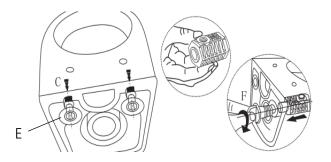
8. Offer the toilet up to the wall, sliding part B into part C and connecting the flush pipe and pan connector into the corresponding pipes in the wall.
