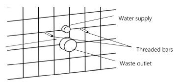
2. Mark the correct lengths for the flush pipe and pan connector (supplied with the concealed cistern).
