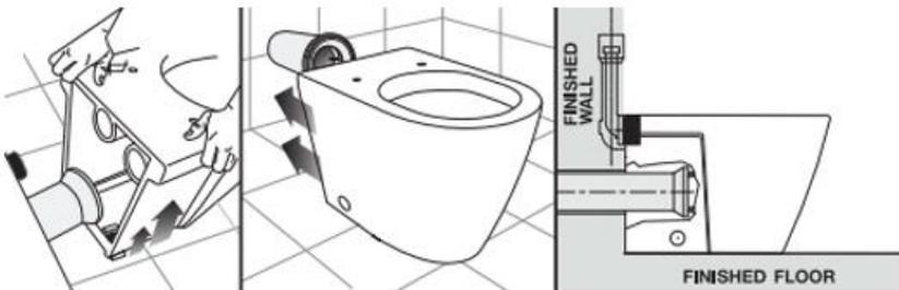
7. Ensure the pan is level and then secure it to the fixing brackets using the pan fixing screws and washers provided. Fix on the cover caps and seal the base of the pan using silicon sealant.
