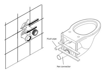
3. Cut the flush pipe and pan connector to the correct length.
