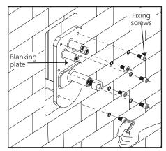
6. Check to ensure that the o-rings are firmly secured in the back of the valve body. If the o-rings are damaged or not seated correctly, the valve body will not seal with the ARMERA dock and leaks may occur.
