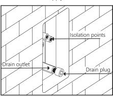
5. Remove the blanking plate from the ARMERA dock. Keep the fixing screws to one side.
