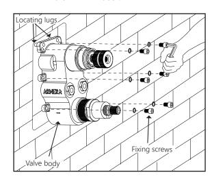
8. Switch on the water supply and check for leaks. Test the water temperature from one of the outlets using a thermometer.
