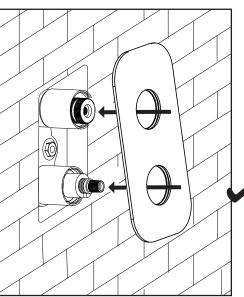
11. Seal the plate to the tiles using silicone sealant. Ensure to leave the channel at the bottom of the plate free of silicone. If a leak ever occurs in the valve, this channel will allow water to escape alerting you of a problem.
