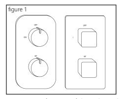
2. Use a thermometer to test the water temperature from one of the outlets. Adjust the temperature by turning the temperature control handle clockwise or anti-clockwise until 38°C is achieved. Remove the handle and re-attach it so it is aligned as shown in figure 1.
