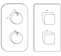
The valve has been calibrated so that 38°C is achieved with the handles positioned as in above diagrams. If water temperature is higher or lower than 38°C, please follow the instructions for recalibrating the thermostat.
