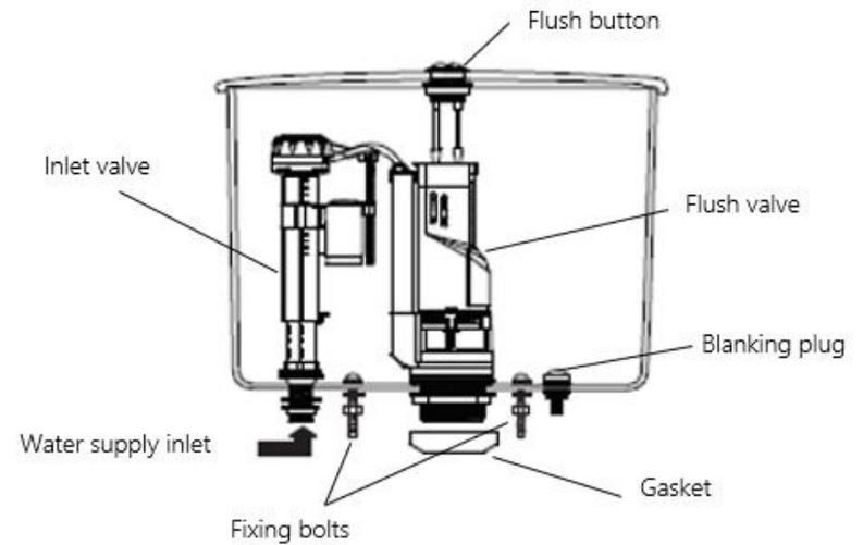
5. Position the cistern onto the pan by centring the gasket on the pan inlet and then secure the cistern in position using the fixing bolts.
