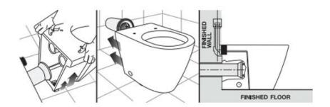
7. Ensure the pan is level and then secure it to the fixing brackets using the pan fixing screws and washers provided. Fix on the cover caps and seal the base of the pan using silicon sealant.
