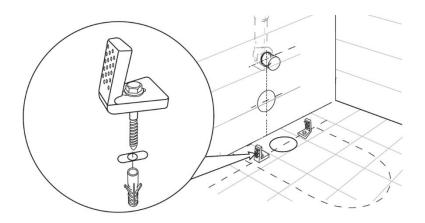
6. Re-attach the flush pipe and pan connector and push the pan back into its final position. Ensure that you make a secure connection with the flush pipe into the water supply and pan connector into the waste outlet. Test for leaks by flushing the toilet before fixing the pan to the floor.
