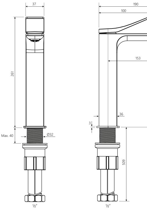
Drill hole diameter: 35mm
