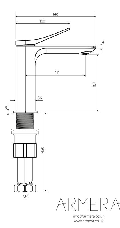
Drill hole diameter: 35mm
