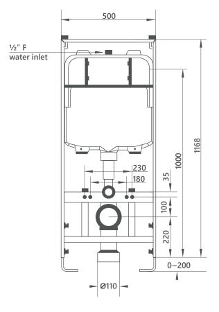
\* NB If outlet pipe runs directly into the wall a minimum depth of 110mm can be achieved by attaching mounting brackets directly to the frame. Please see product instructions for installation detail.
