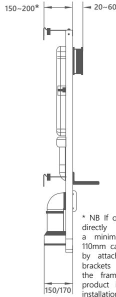
\* NB If outlet pipe runs directly into the wall a minimum depth of 110mm can be achieved by attaching mounting brackets directly to the frame. Please see product instructions for installation detail.
