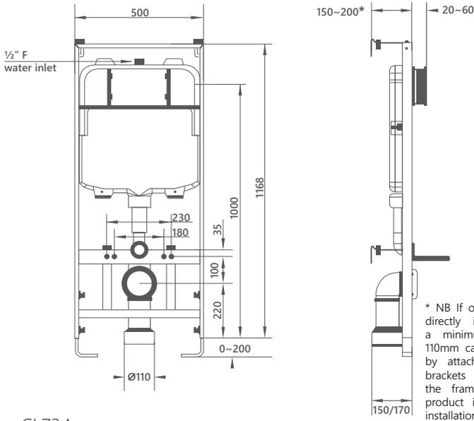
\* NB If outlet pipe runs directly into the wall a minimum depth of 110mm can be achieved by attaching mounting brackets directly to the frame. Please see product instructions for installation detail.
